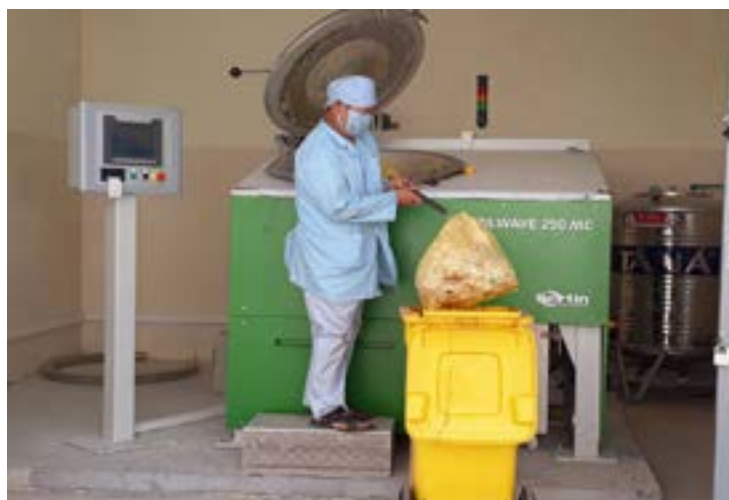
▲ Treating medical waste using microwaves to ensure meeting environmental standards by the General Hospital of Cao Bằng Province
